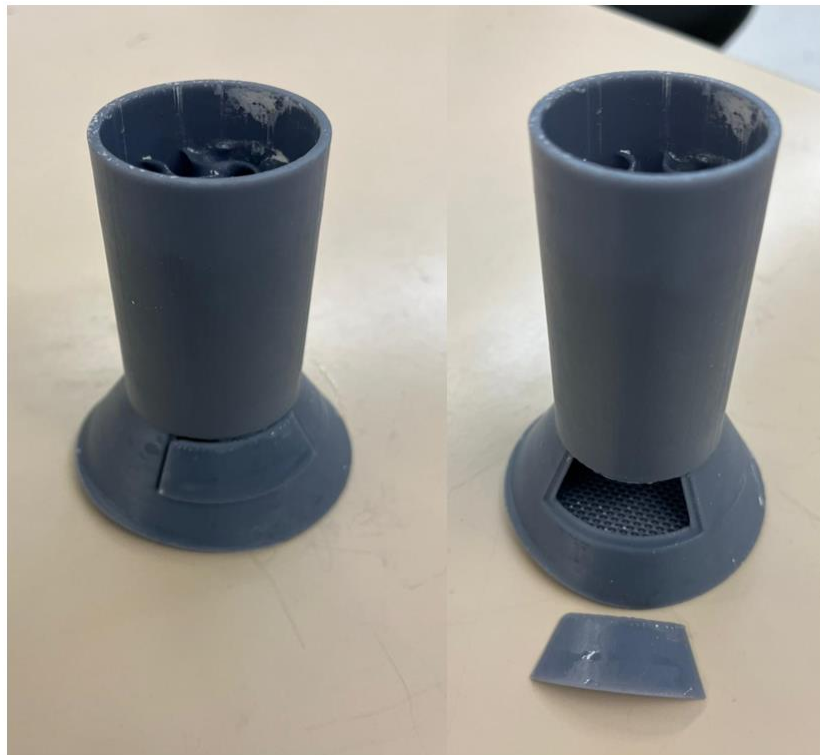
Figure 9: Additively Manufactured (SLA) MicroTRAP device
