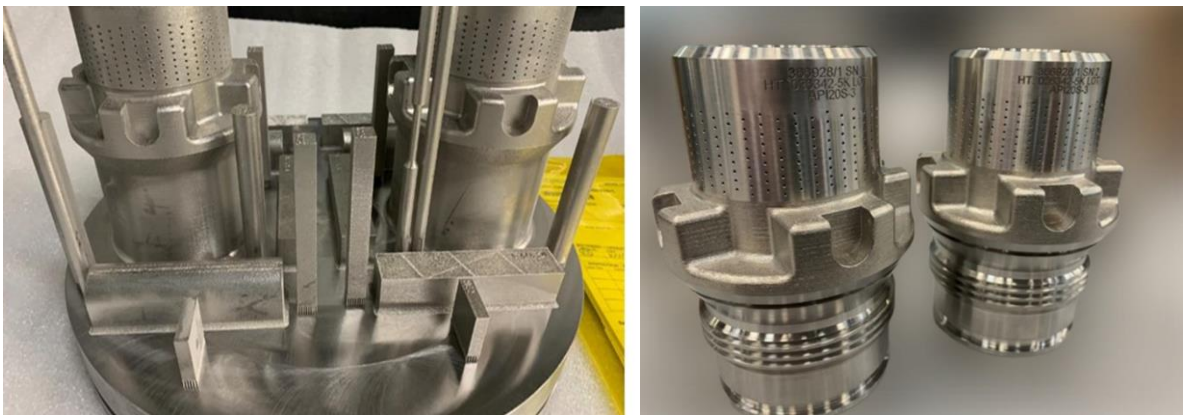
Image 4a & b. (a. Left) Two choke valves, optimized with IMI’s DRAG technology, shown on the build plate after being 3D printed with VELO 3D ’s Sapphire system, and (b. right) the two valves after finishing.
